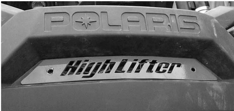
4. Using the two 5/16 x 1" button head bolts, 5/16" washers and 5/16" lock nuts connect the plate.
