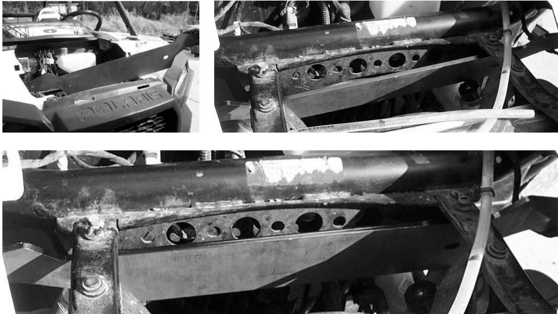
8. Insert the 10 x 70mm bolt through the bracket, placing a 10mm washer between the bracket and the shock mount.
