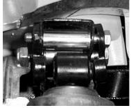
8. Connect the top of the shock between the two lift brackets using a 10x65 hex bolt and 10mm lock nut.
