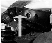
5. Insert one 10x 65mm hex bolt thru one of the right lift brackets, and then place the small rear spacer into the stock shock mount location. Insert the bolt thru the shock mount and spacer.
