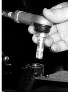
5) Connect the tie rod ends to the new tie rods. Make sure to notice the grooved end of the new tie rod. This end has the left handed threads. This will be connected to the tie rod end that is attached to the knuckle /hub assembly.
