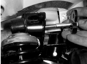
6. Next, place one left lift bracket onto the bolt and fasten it with a 10mm lock nut.
