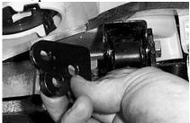
7. Now, place the large spacer into the frame, between the two lift brackets, and connect them using the 5/16 x 2 1/5 hex bolt. Secure it using a 5/16 lock nut.
