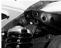
NOTE: VERY IMPORTANT WHEN DISCONNECTING THE SHOCK FROM THE FRAME DO NOT LET THE CONTROL ARM DROP SUDDENLY. THIS CAN CAUSE THE AXLE TO PULL OUT FROM THE DIFFERENTIAL.
