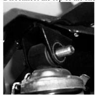
8) Insert the small spacer in the shock mount tab and place the Front Lift Brackets on either side of the shock mount tabs. Secure the brackets and spacer using 10 x 60mm hex bolt and 10mm lock nut.
