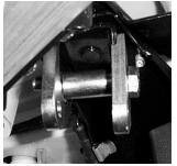
NOTE: If the brackets do not fit just right the Stock Shock Mount is Adjustable and can be moved. You may need to adjust it to make the brackets fit properly.
