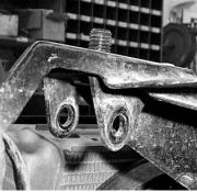
9) Connect the top of the shock to the lift brackets using the 10 x 60mm hex bolt and 10mm lock nut.
