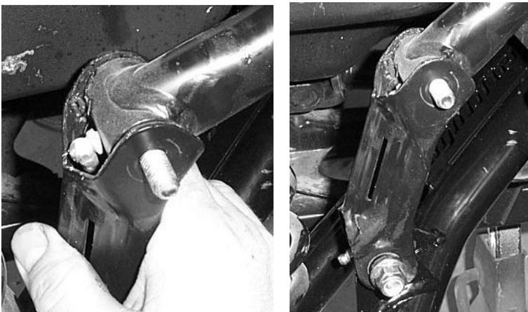
19. Attach brake lines to the new trailing arm by using the factory hardware and zip ties provided in the kit.
