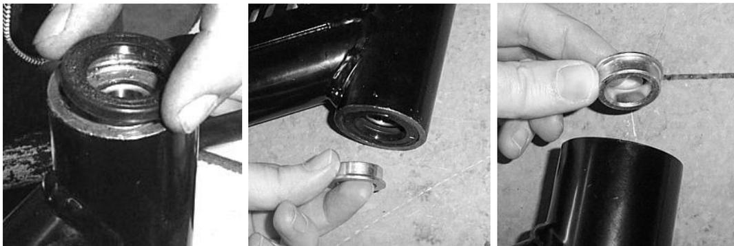
13. Remove the factory bushings and sleeves from the sway bar mount in the stock trailing arm and insert them into the sway bar mount on the High Lifter Trailing Arm.
