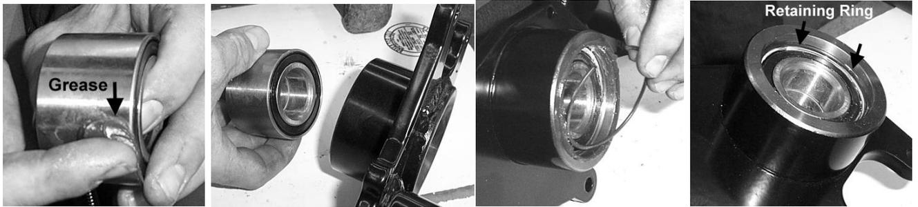
12. Now, install the 4 bearings, 1 sleeve, and 2 seals on the frame end of the trailing arm. This will be difficult!!! Start by installing two of the bearings in one side of the arm. Then insert the sleeve in the opposite end. Next install the remaining bearings. Place the seals and factory spacers on both ends.
