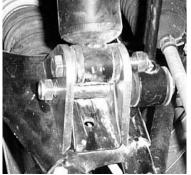
9) If you have not done so already, disconnect the top of the stabilizer rod from the stabilizer bar. Remove both rubber bumpers.
