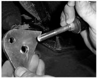
8) Insert the Large Spacer between the shock mount tabs and insert the 10x110mm bolt through the shock mount tabs and spacer. Fasten brackets and both bolts with the 10mm lock nuts.
