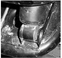
5) Insert the Large Spacer into the shock mount.
