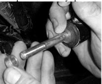
7) Insert the 10x110mm bolt through the bottom hole on the lift bracket.
