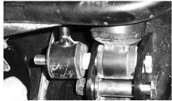
10) Place the large factory washer next to the stabilizer rod eyelet and fasten tight with the 10mm lock nut.
